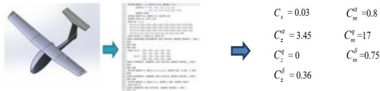
Fig. 3.23. Determination of UAV stability derivatives using DatCom software
