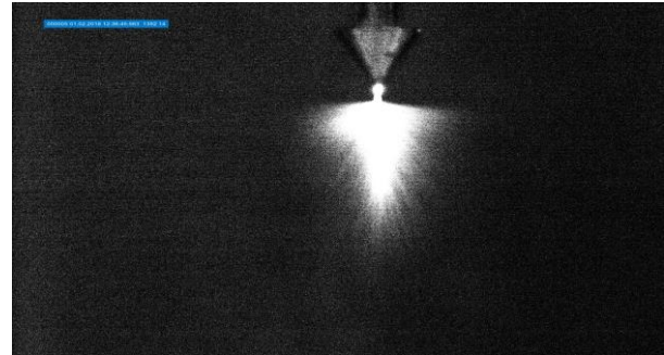
b) Laboratory generated Corona discharge (Data Set 2)
